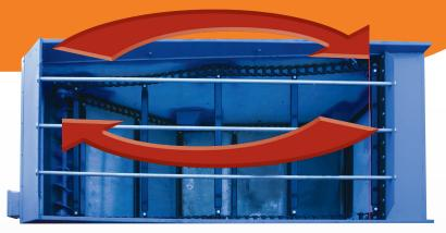
Feed enters the heavy-duty auger at the left and right sides of the mixer and keeps the feed higher in the center as it blends. The feed spreads as it is carried towards the rear by the return chain. The heavy-duty chains with  $1\frac{1}{2}$  high paddles blend the whole batch end to end. This insures very accurate mixes.
