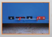
Convenient chain adjustment is outside at bottom of box
